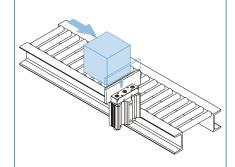
Tough type of stopping a large-load work carrier at a fixed point, and for the straggle of a number of work carriers, etc.
