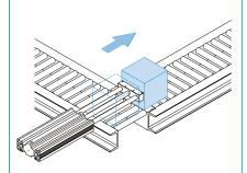
Long strokes available, the highly precise pushing work transfers and places a work carrier and changes the direction.
