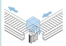
Special design which stands the large one-sided load. Lifts the work carrier at a fixed point not changing the posture.
