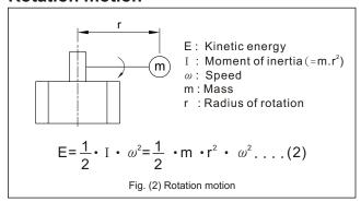
In the case of the kinetic energy for linear motion, the formula (1)shows that when the velocity v is constant, it is proportional to the mass m. In the case of rotation motion, the formula (2) shows that when the angular velocity is constant, it is proportional to the moment of inertia.
