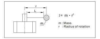
This formula represents the moment of inertia for the shaft with mass m, which is located at distance r from the shaft. For actual loads, the values of the moment of inertia are calculated depending on configurations, as shown on the next page.
