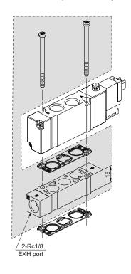
Individual SUP spacer assembly + Individual EXH spacer assembly
