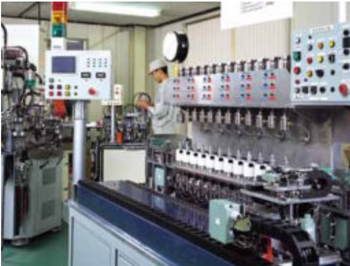
Automatic Cupla inspection system
