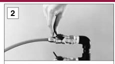
Turning down the lever opens the valve and allows the fluid to flow. (The turned-down lever works as a sleeve stopper and prevents disconnection.)
