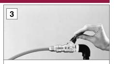
When the lever is pulled up, residual air in the plug is purged without unpleasant noise and kick back on disconnection. In this stage, the socket valve is still closed.
