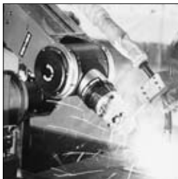
Piping to work clamping device on welding robot
