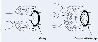
② A HSP Cupla has a backup ring. Insert an O-ring in the place shown in the figure. If Cupla connection/disconnection is hard and not smooth after the O-ring has been replaced, apply a little grease to the O-ring.
