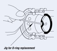
2 After removing the O-ring, wipe the groove clean with a cloth.
