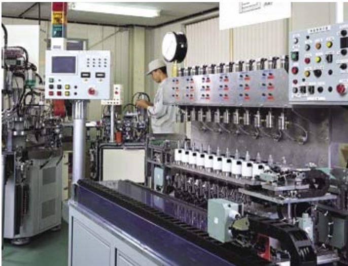
Automatic Cupla product inspection system
