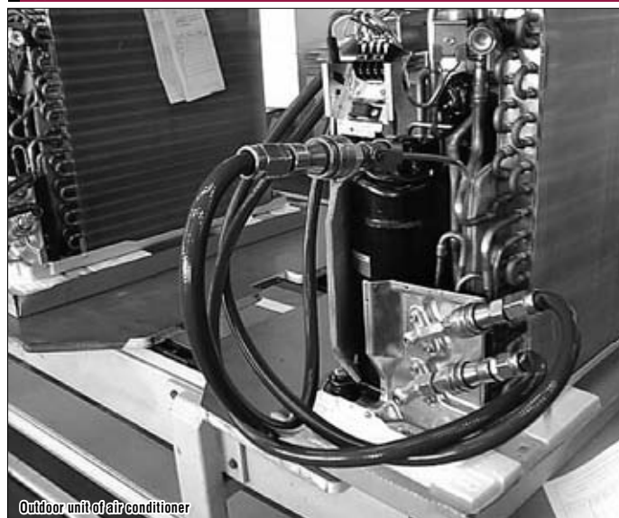
Outdoor unit of air conditioner
