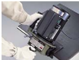
Chamfering steel plates
